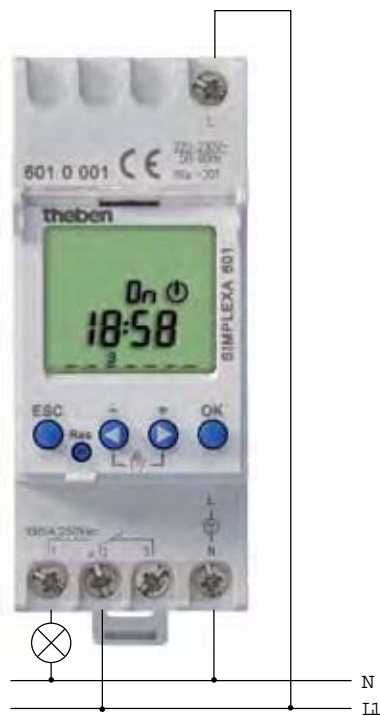
SM PLEXA 601 - Connection diagram
