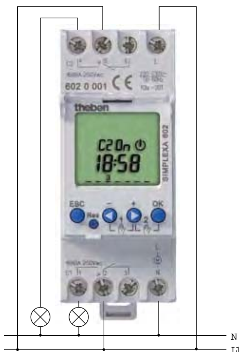
SM PLEXA 602 - Connection diagram
